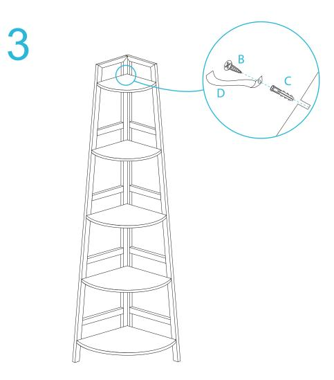
Attach the other end of the safety straps (D) to the wall using 2x wall plugs (C) and 2x 25mm scews (B). Tighten with a screwdriver. You're done, enjoy!
