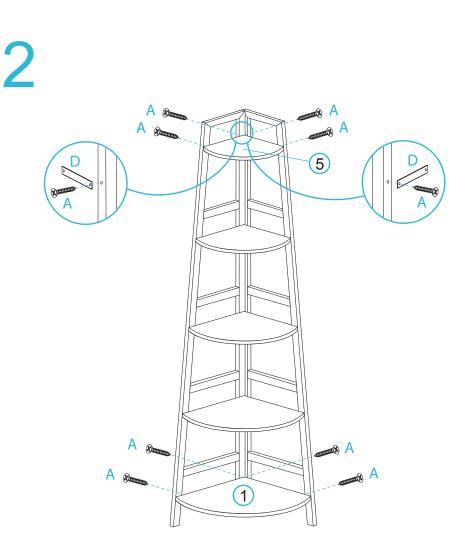
Attach shelf panels [2], [3] and [4] to the main unit as shown and secure with 12x 50mm screws (A). Tighten with a screwdriver.
